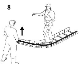
Bend the LifeLadder to distribute tension. Example: One person stands on the ladder while another person lifts up the end of the ladder. Tighten plastic nuts again.
