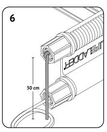
Tighten the knot. Cut excess rope 30 cm from knot. Repeat steps 4-6 for the other three ropes.
