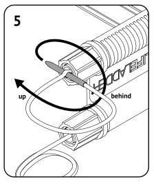
Use the Splice Needle to put the rope through itself.
