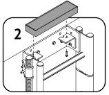
Unpack and fix LightUnit to the Supports with 2x Button head screws (included).
