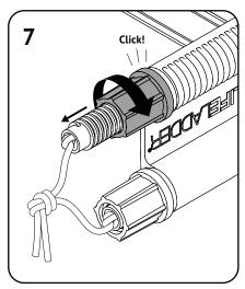
Tighten plastic nuts by hand. Tie ropes together with an ordinary knot.
