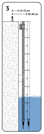
Tighten Clamps. Position Handhold 15-25 cm from quay wall ~ 30-40 cm from center of LifeLadder step.
