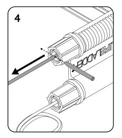
Pull rope **as hard as possible** (particularly important with long ladders). Then, pierce rope with Splice Needle next to the plastic nut.
